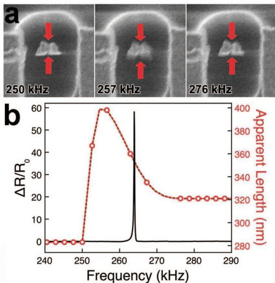
**Figure 3.** (a) Series of scanning electron micrographs of a device during AC actuation (frequency indicated), showing apparent blurring when resonance is met. The red arrows indicate the apparent length of the device at each frequency. (b) Plot of resonance peak measured by transport (black) and the apparent length of resonator measured directly from imaging (red).
