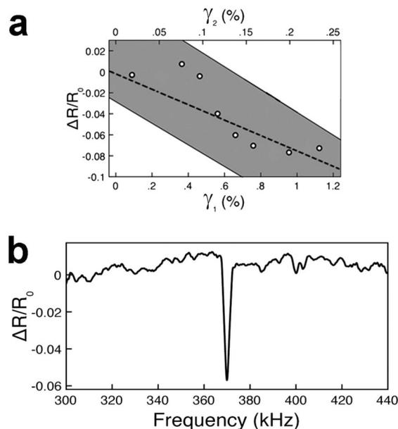
**Figure 4.** (a) Quasi-static measurement on a second device, demonstrating a decrease in resistance with added strain. The elements are the same as those described in Figure 1b. (b) Differential resistance vs. applied actuation frequency on the same device, yielding a peak that agrees in direction with the quasi-static measurement.
